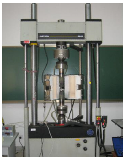
Figure 14. SDM100 electrohydraulic servo fatigue test machine.
