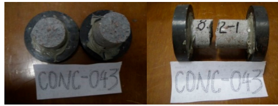
Figure 2. Failure under tensile stress.
