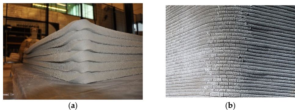
Figure 5. Printing quality problems with rectangle/square nozzle section: (a) twisted filament [108]; (b) tearing and cracking of printed curve layers [109].
