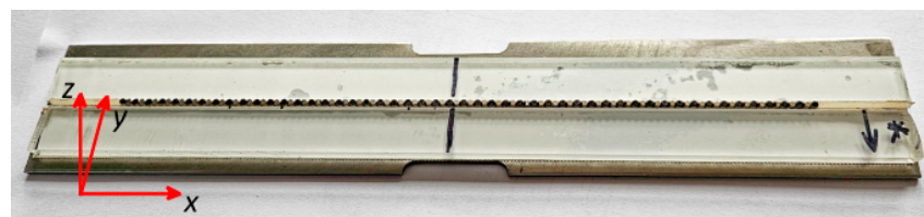
Figure 3. An array of permanent magnets as the magnetizing system. The samples are magnetized by moving the system along the y -axis.
