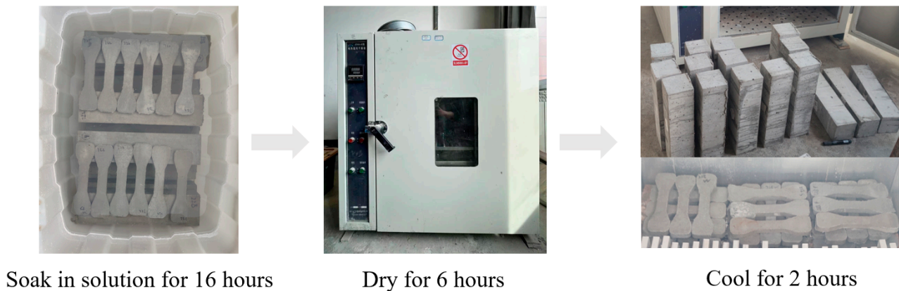
Figure 4. Schematic diagram of dry–wet cycle.
