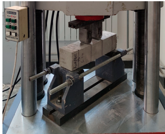
Figure 6. Four-point bending test device.
