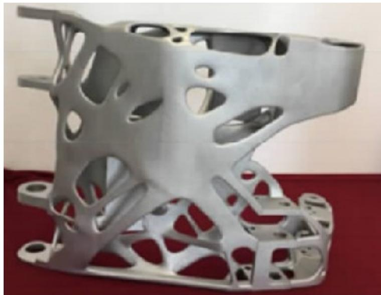
**Figure 12.** Hinge arm printed by LPBF process [27].
