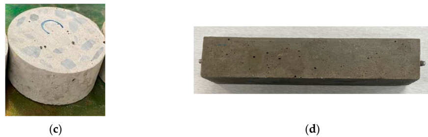
Figure 4. Photos of (a) axial compression, (b) splitting tension, (c) water absorption, and (d) drying shrinkage test samples.
