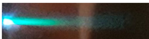
Figure 2. The self-emission of a plasma plume generated by 600 fs pulses of 4.4 \pm 0.2 mJ energy hitting the copper target surface as seen by a CCD camera.
