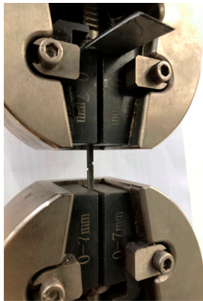
Figure 6. Actual tensile–shear testing process of specimen in the machine.
