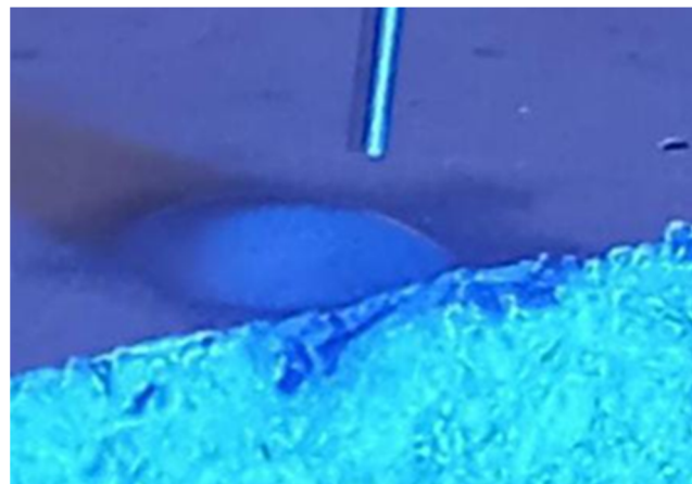
Figure 7. Illustrative image of the ultrapure water droplet on the surface of the cementitious composite and its absorption into the upper layer of the sample.
