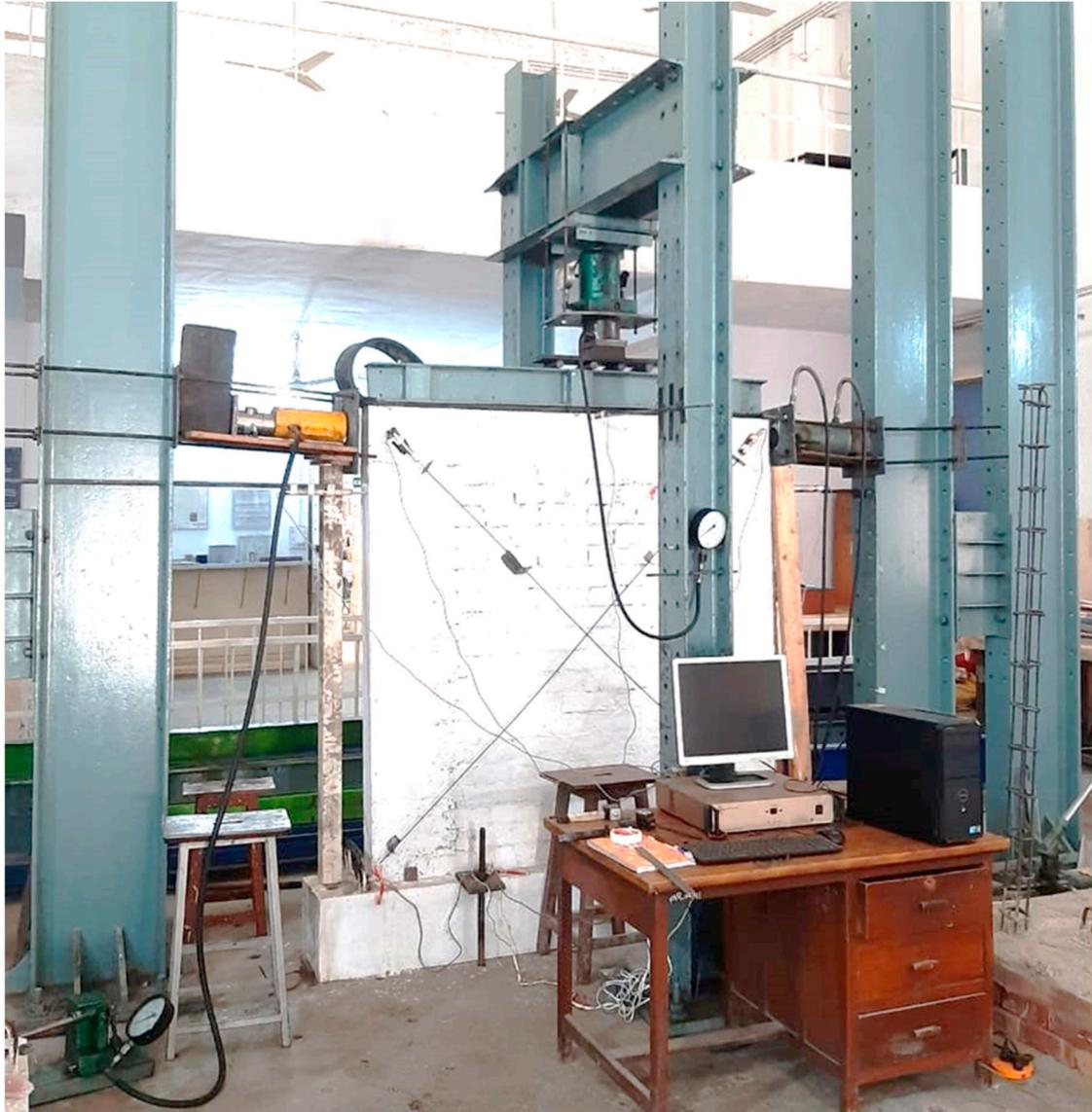
**Figure 2.** CM wall test setup and instrumentation [38].
