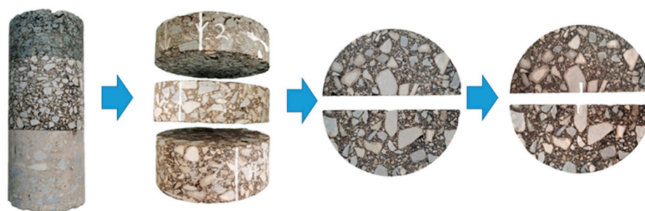
Figure 1. Core sample processing procedure.
