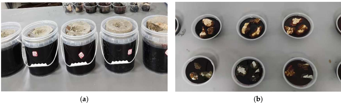
Figure 1. (a) rock penetration test immersion; (b) rock strength test immersion.
