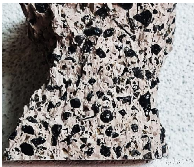
Figure 5. View of the geopolymer mortar breakthrough.
