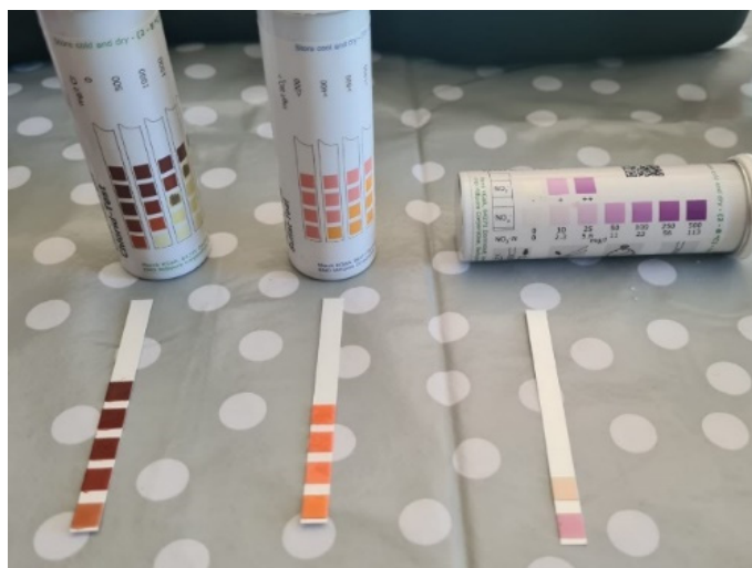
Figure 10. Assessment of salt content carried out on 20 samples taken from various places in the building (photo by authors).
