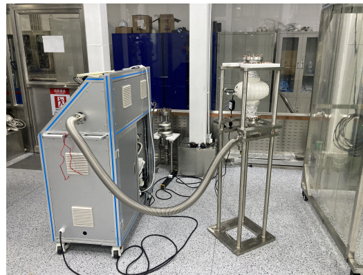
Figure 7. A 1.3 GHz single-cell cavity undergoing the two-step baking process.
