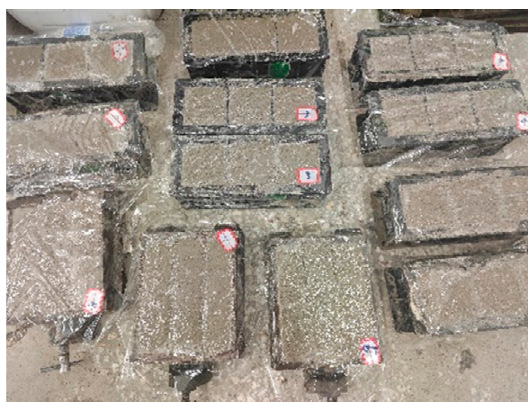
Figure 4. Cast-in-place test block.
