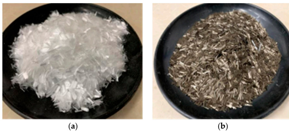
Figure 1. (a) Polypropylene Fiber; (b) Basalt Fiber.
