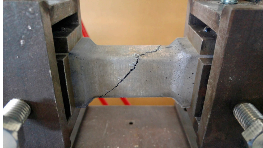
Figure 9. Destroyed specimen mounted in the apparatus stand after the torsion test.
