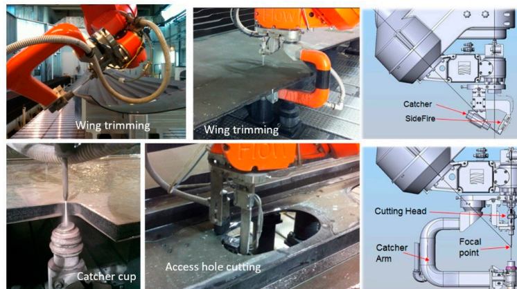
Figure 49. Focal point C-frame end effector for composite trimming.
