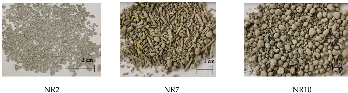
Figure 11. Examples of artificial aggregate granules that were made.
