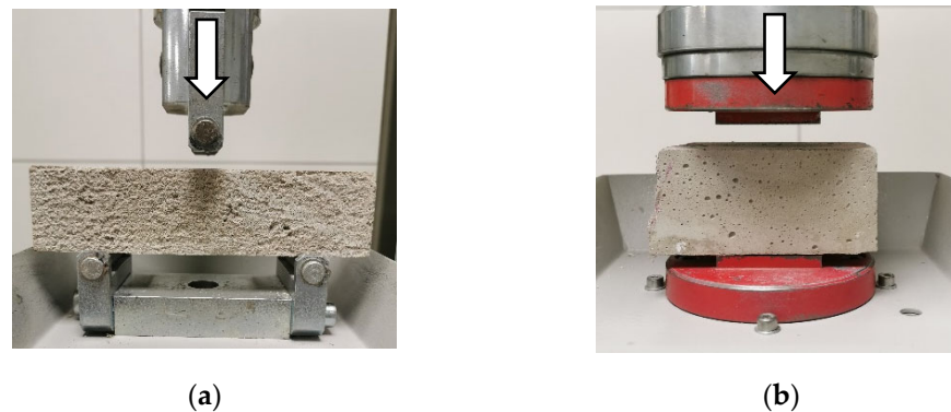
Figure 8. Flexural (a) and compressive (b) strength tests of 3DPC prisms [42,43].
