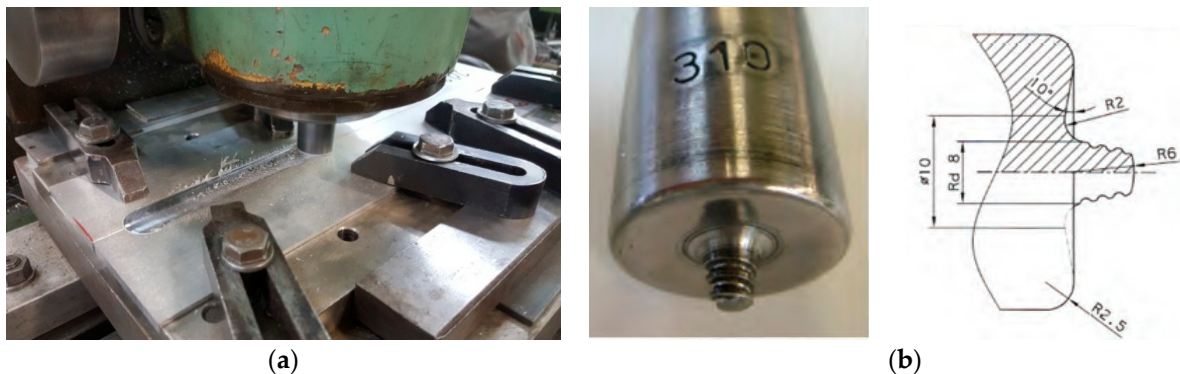
Figure 1. (a) Conventional milling machine for FSW and (b) geometry of FSW tool.
