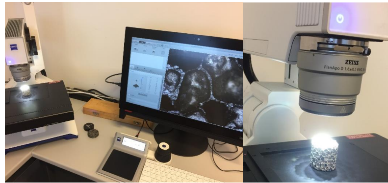
Figure 7. Microscope investigation to reveal the size of void inclusions and their deviations.
