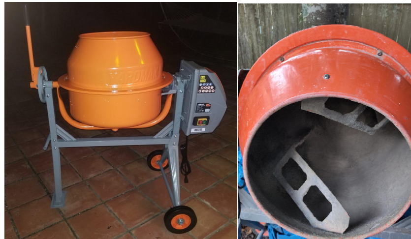
Figure 5. Mixing machine, exterior and interior view with the blades.
