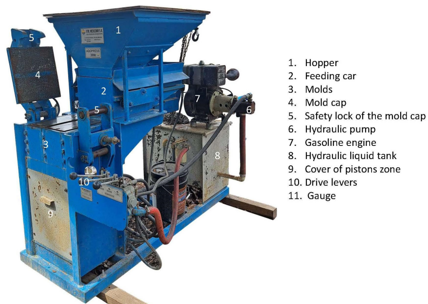
Figure 6. Adopress 3000—CEB Making Machine and its parts.
