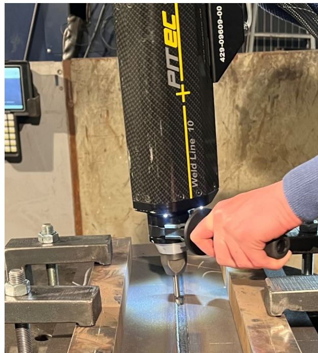
Figure 4. HFMI treatment of welding joint.
