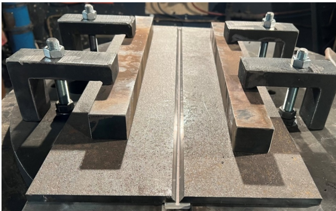
Figure 2. Test plate with ceramic backing on the welding robot bench.
