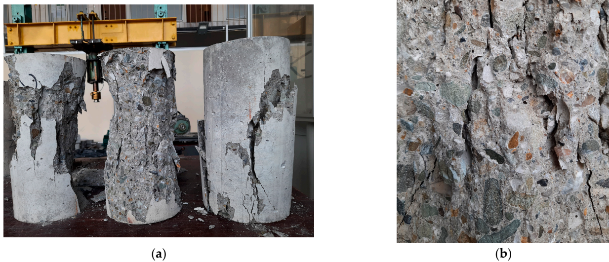
Figure 6. Examples of normal-weight concretes after failure at compression: (a) Typical failure method; (b) typical fracture pattern.
