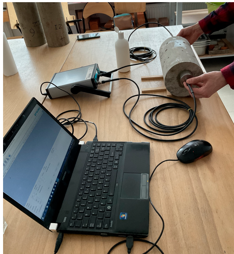
Figure 5. Testing equipment used for measurements of ultrasonic pulse velocity.
