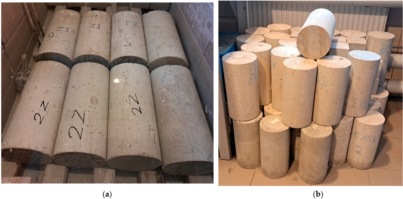
Figure 2. Test specimens cured in water (a) and in air (b).
