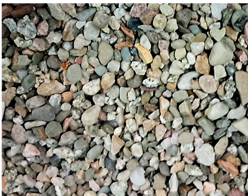
Figure 1. Normal-weight coarse aggregate 4/16 mm was used for composite preparation.
