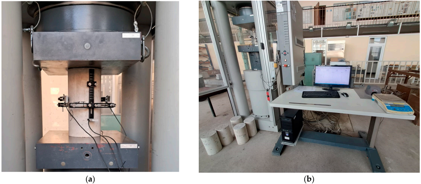
Figure 4. Testing equipment used for measurements of static secant modulus of elasticity: (a) a concrete cylinder under compression; (b) automatically controlled compressive testing machine.
