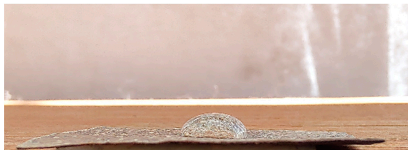
Figure 2. Water drop deposited on the surface of the SCB sample.
