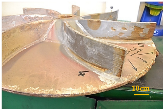
Test rotor blade with WC Co CrC Ni coating (HVOF) HV_{0.2} = 1195
