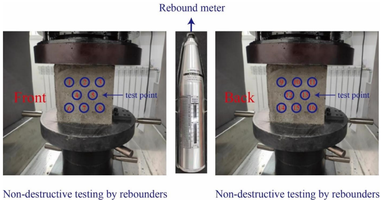
Figure 8. Rebound value test of recycled concrete.
