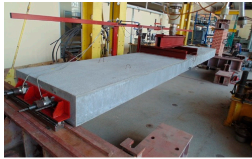
Figure 9. View of tested slab and load stand.
