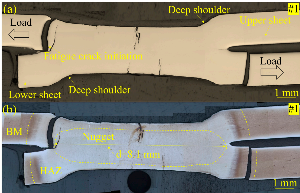
Figure 9. Micrographs of the Zn-coated steel RSW joint of tensile-shear specimen #1 after a fatigue test: (a) without chemical etching and (b) with chemical etching.
