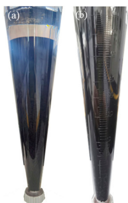
Figure 7. (a) PPH and (b) terpeneol system slurries after 30 days of standing.
