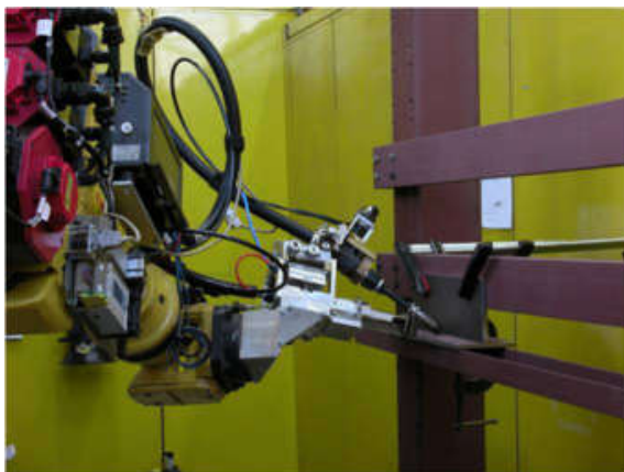
Figure 26. A view of the experimental stand of the LHW process of T-joint of EH 36-grade steel plates 12.0 mm thick and the welded joint macrostructure [12].
