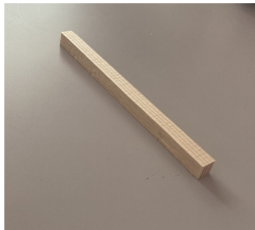
Figure 1. Final specimen dimensions: 10 mm × 10 mm × 150 mm.
