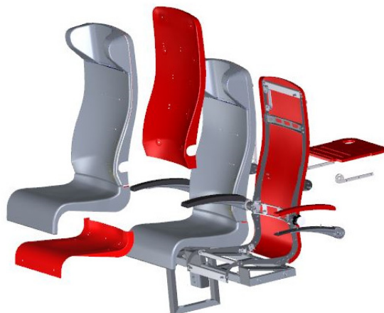
Figure 1. Visualization of a railway seat with polymer composite elements marked in red.
