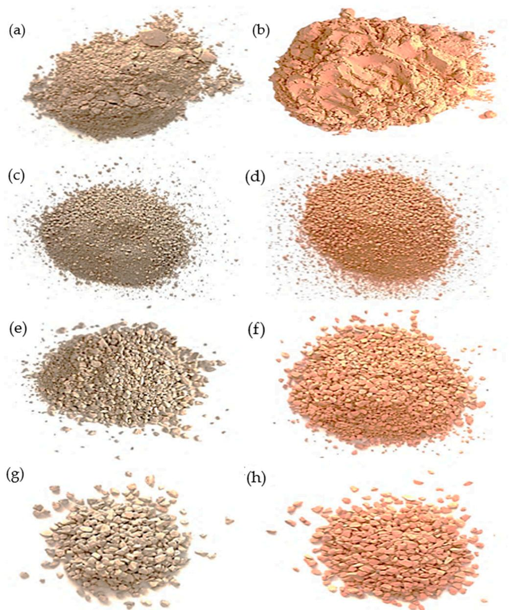
**Figure 3.** Diatomite: (a) diatomite powder, (b) diatomite powder after calcination, (c) granules, (d) granules after calcination, (e) 0.5–3 mm aggregate, (f) 0.5–3 mm aggregate after calcination, (g) 2–5 mm aggregate, and (h) 2–5 mm aggregate after calcination.
