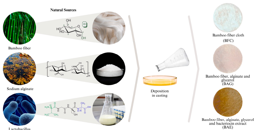
Figure 1. Diagram of the biocomposite production through natural sources and the plate deposition method.
