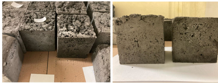
Figure 2. Prepared test samples with PCM additive (overview photo) (samples measuring 10 \times 10 \times 10 cm).
