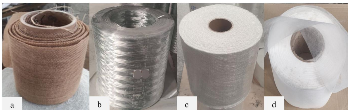
Figure 1. (a) Kenaf fibres (woven); (b) E-glass fibres (direct roving); (c) E-glass fibres (woven); (d) surfacing veil.
