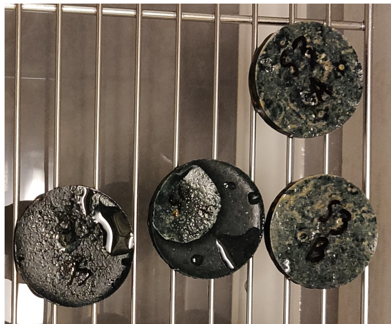
Figure 5. Samples for composition S05M8 and S08M8 exposed to 98% relative humidity.
