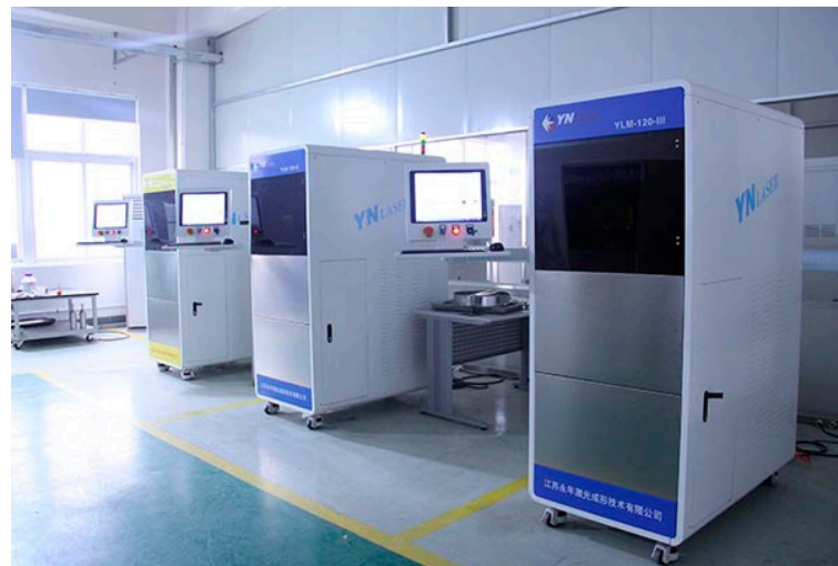
Figure 2. YLM-120 SLM machine used in this work.
