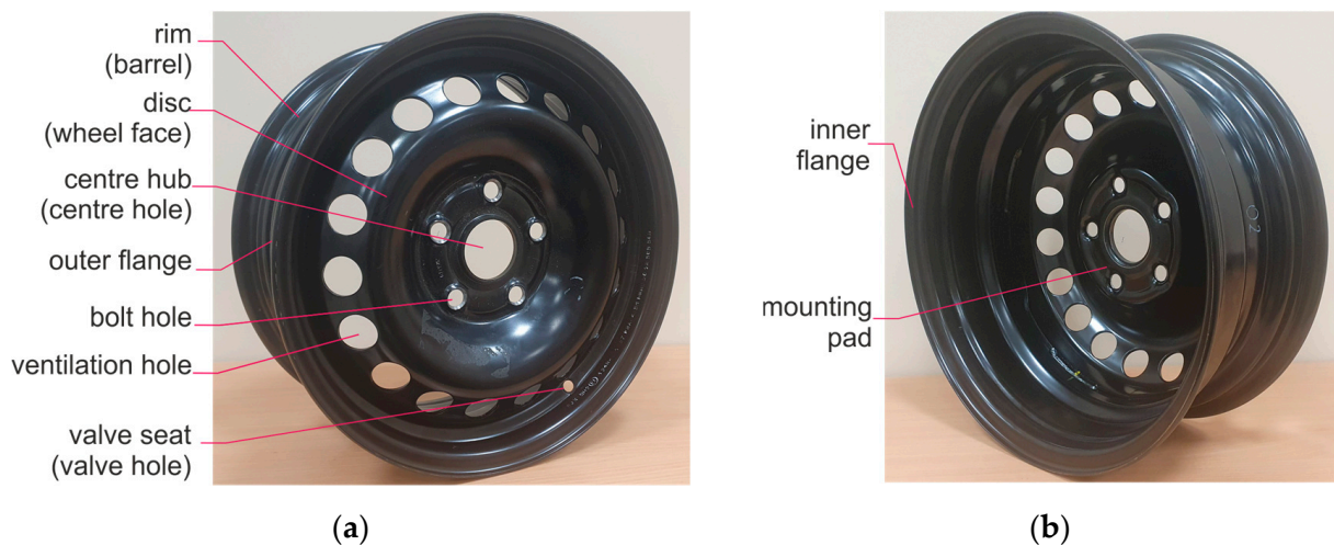
Figure 1. View of a steel automotive wheel rim: (a) Outer view; (b) Inner view.
