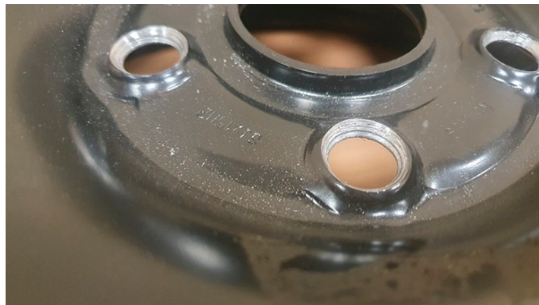
Figure 19. Degradation of bolt holes after 40 h of the fatigue test with rusty hub use for the new rim from ARM.
