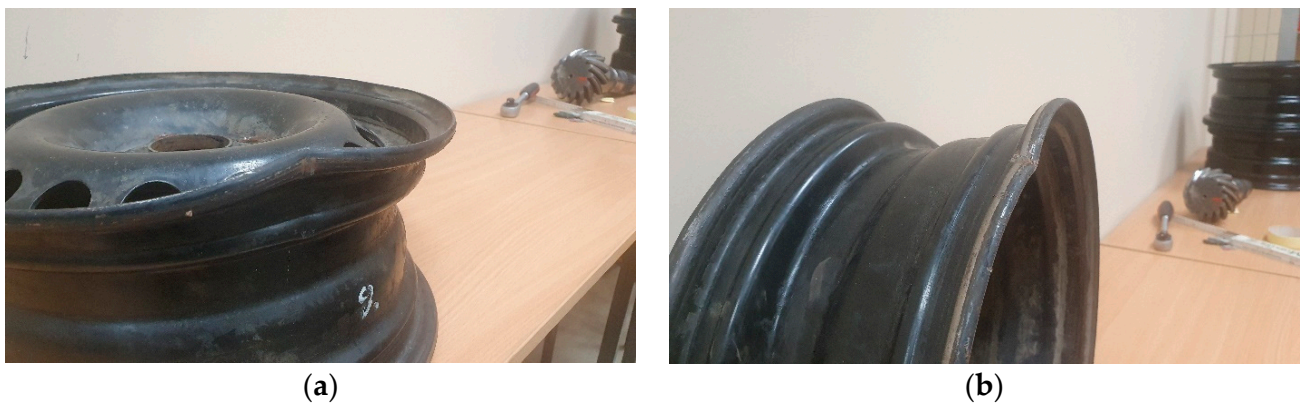
Figure 32. View of rim: (a) After it hit a curb; (b) Further six months of operation on partially paved forest roads.
