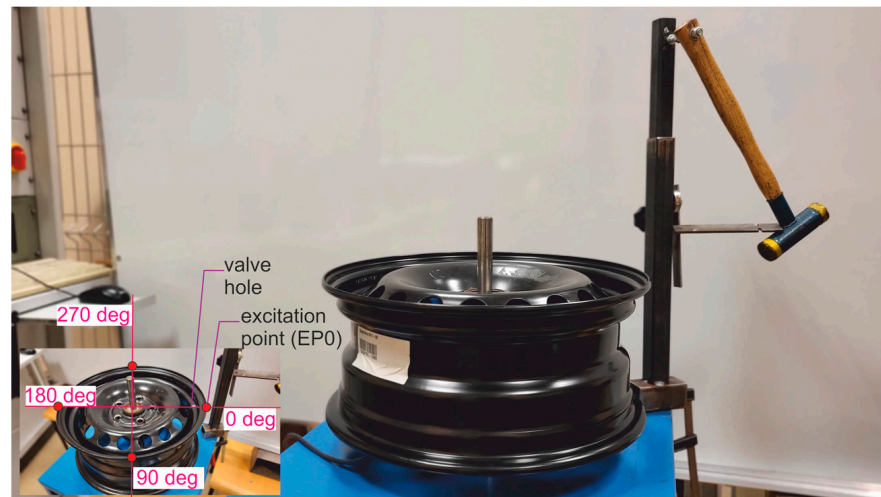
Figure 6. View of the mechanical part of the measurement system for EMA with vibration excitation points (EP) marked.
