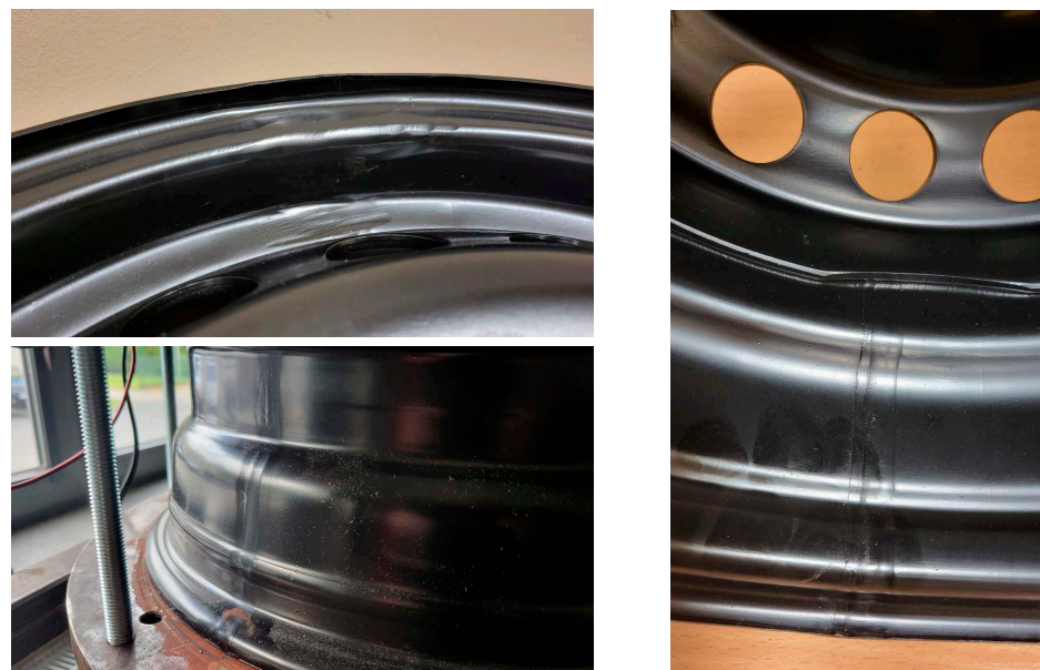
Figure 23. Views of imperfections of the second rim from LCM.
