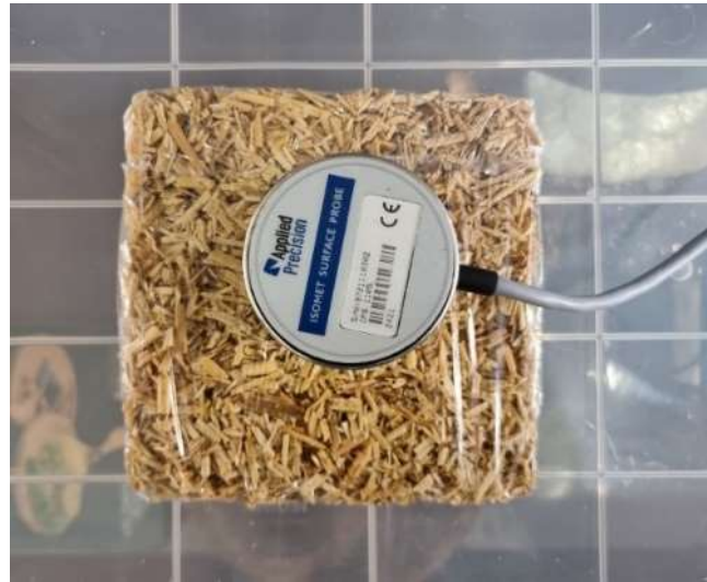
Figure 5. Measuring thermal conductivity with a disk probe.
