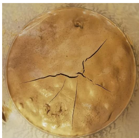
Figure 9. The form of failure of filter cake air tightness in constant air pressure.
