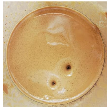
Figure 6. The failure morphology of filter cake in high air pressure.
