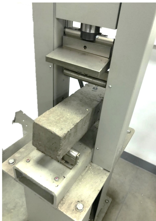
Figure 5. Flexural strength test setup for a beam specimen.
