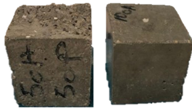
Figure 3. Samples of concrete blocks.
