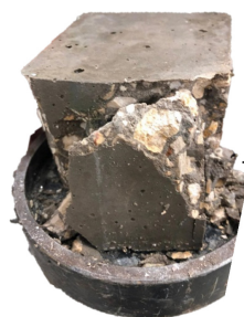
Figure 4. Failure of the concrete block under compression test.
