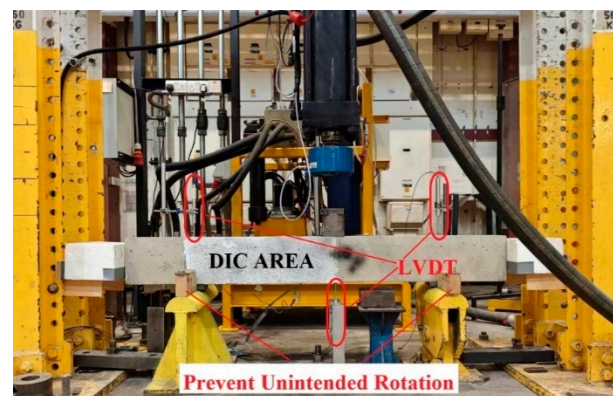
Figure 3. Three-point bending test setup of beams.
