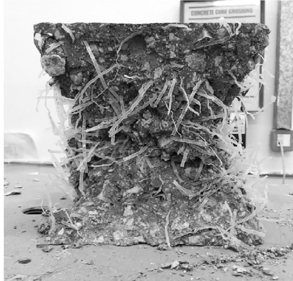
Figure 8. Deformed fiber-reinforced cube after failure [82].
