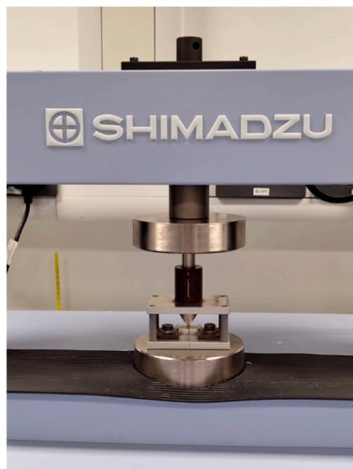
**Figure 2.** Shimadzu universal testing machine with a sample loaded in the test rig—3-point bend test jig.
