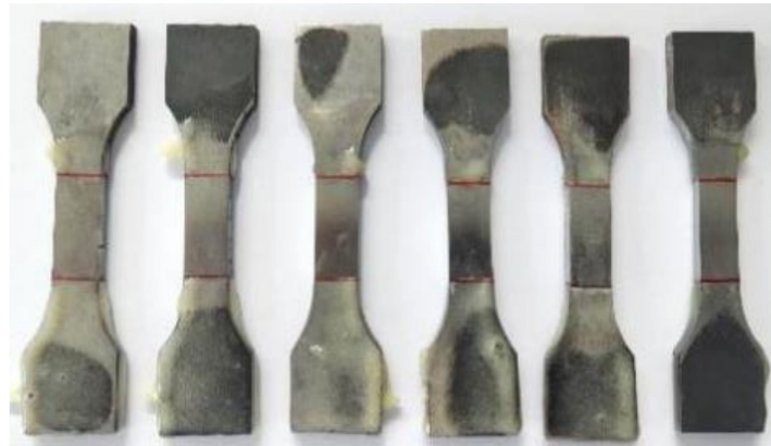
Figure 2. Q690 high-strength steel weldment specimens (the area between the two red lines of the specimen is the part for the electrochemical hydrogen charging).
