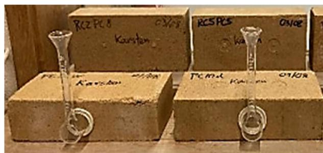
**Figure 4.** Low-pressure water absorption test.
