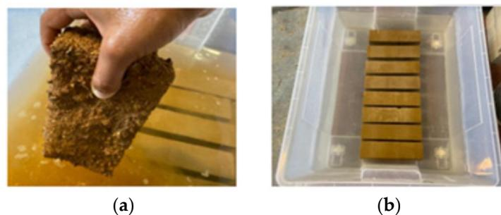
**Figure 12.** Blocks' immersion absorption: (a) UCEB; (b) SCEBs with different types of stabilisers (RC, PC).
