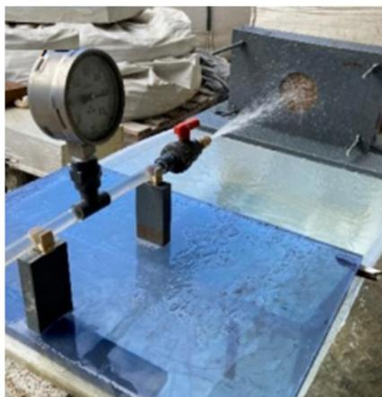
**Figure 6.** Water erosion resistance test.
