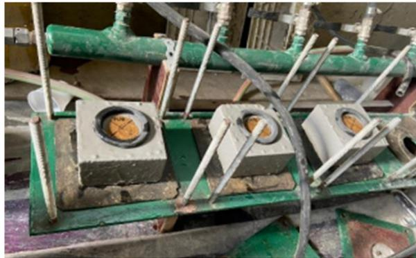
**Figure 5.** Water permeability test.
