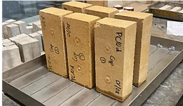
**Figure 3.** Capillary absorption test.
