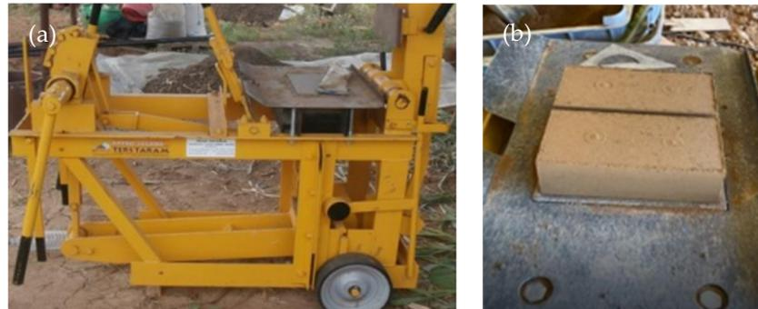
**Figure 2.** Compressed earthen block production: (a) manual press; (b) blocks just after being compressed.
