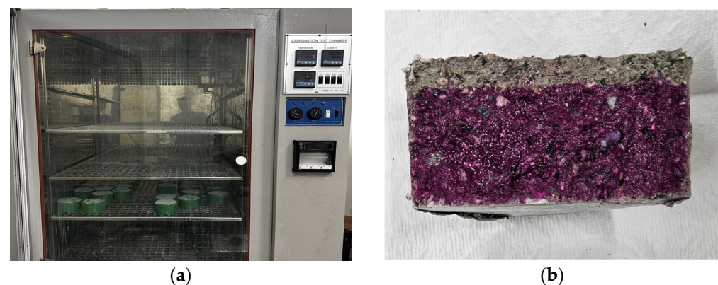
Figure 5. (a) Accelerated carbonation chamber and (b) carbonation depth measurement.
